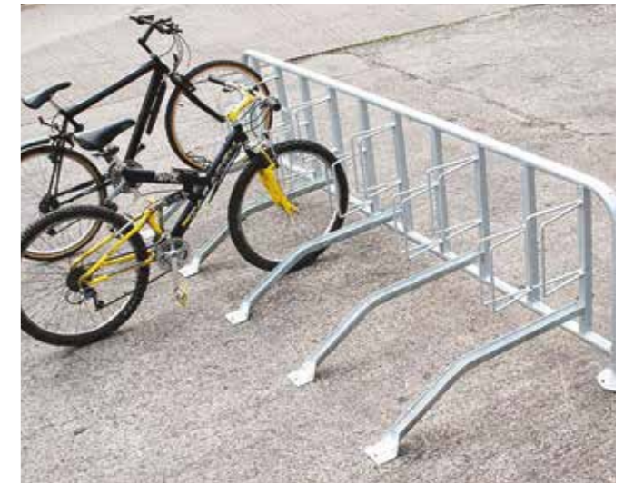
Ramped stands These, like wheel racks, must be avoided as they provide no locking points for a bicycle frame and provide no support. They can also damage bicycle wheels.
