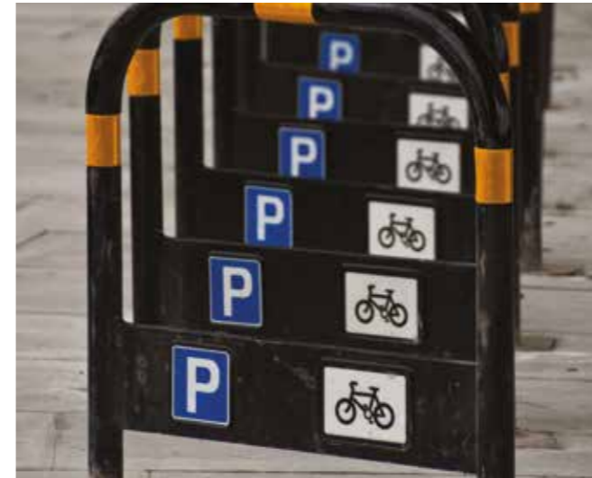
Sheffield stand Parks 2 bicycles and represents one of the most cost effective cycle parking solutions. Supports different types of cycles. Can lock both wheels.
